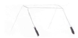
Cut 1" conduit into 2-2.5' lengths and pound them into the ground the same angle as the leg poles. Stick the leg poles inside the 1" conduit. Some have drilled a hole and either used a bolt or wire to fasten the leg pole inside the 1" conduit. I thought the cage might still sway at the top in windy climate, but many of my clients have said this works for them. Or use rebar and tie the leg pole to the rebar.
